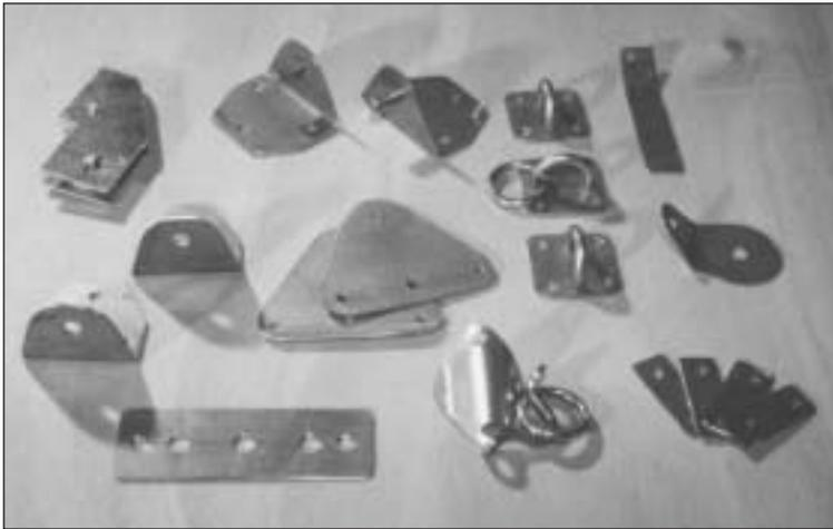
A set of homemade Firebug deck fittings
