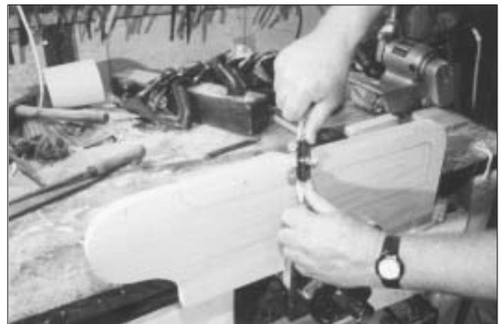
Using a spokeshave on the rudder blade
