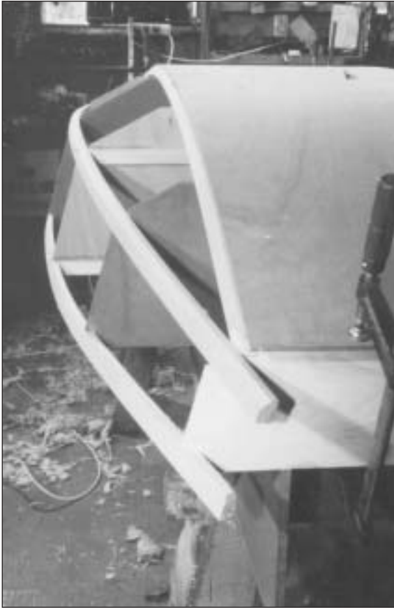
10 9mm ply bottom going on
