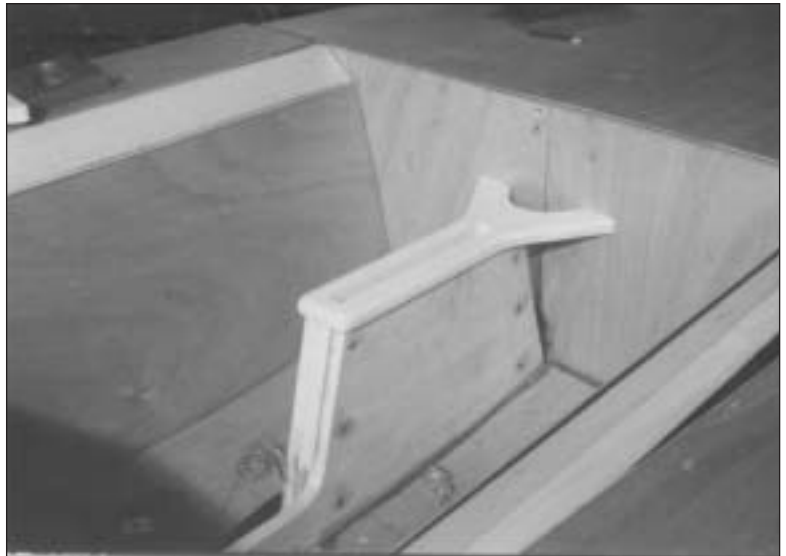
16 Carlins and centre case top fitted
