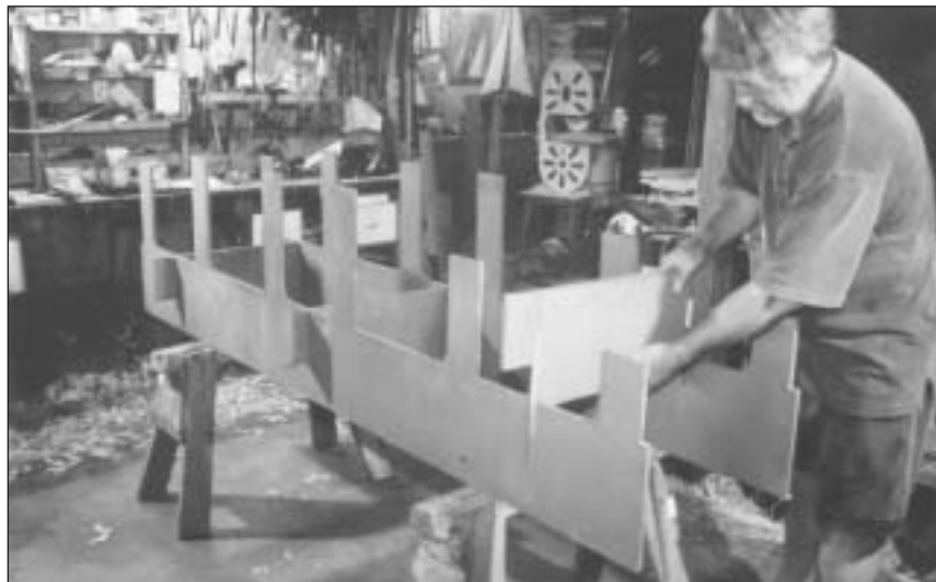
6 THIS building jig slots together.
