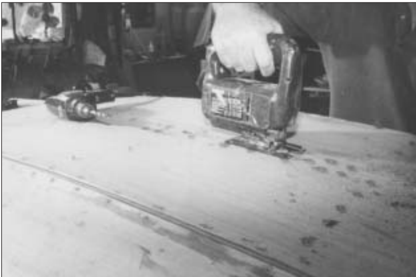
11 Cutting the centrecase hole
