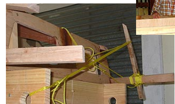
Ross Venner's 'Spanish Windlass' - cords and levers used in lieu of conventional clamps. Cheaper too!
