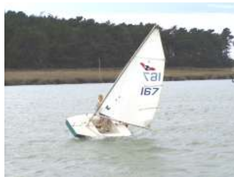
This Firebug is making the same mistake. In heeling, you can see how the bow curve will want to turn the bow into the wind
