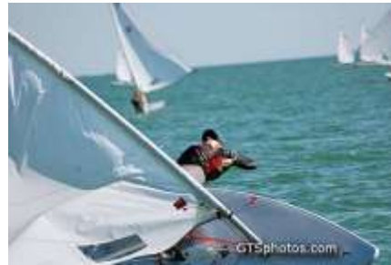
Sail looks too full for the conditions and the skipper is fighting to keep the boat on course. Again ease the main and go with the gust
