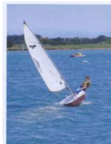
This Firebug is making the same mistake. In heeling, you can see how the bow curve will want to turn the bow into the wind
