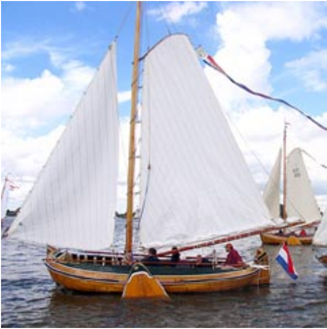
One of the smaller boats showing leeboards and rig.
